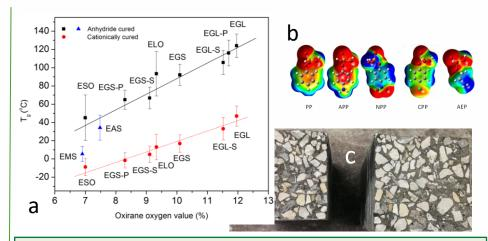
a) Polymer glass transition as a function of soybean oil monomer oxirane conc.; b) Charge densities of ligands for dielectric composites; c) Smooth, cohesive failure mode for low ASR, higher tensile strength concrete
